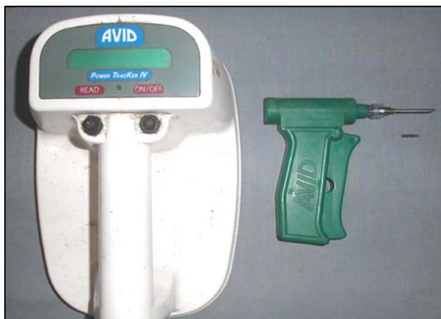
Figure 9: PIT tag scanner and gun with needle. Note the small plastic bar coded PIT pictured below the needle.
