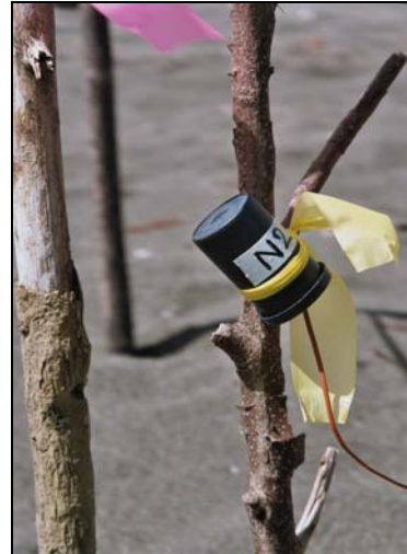
Figure 5.12 Thermocouple covered with a film Canister and fixed on a stick next to the nest (photo by Sue Furler, 2004)
